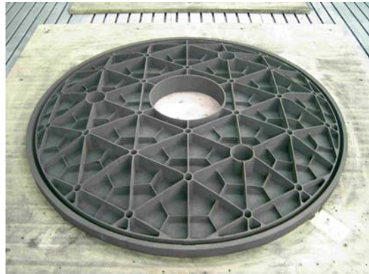
Fig.8b : Greenbody manufacturing backside completed
