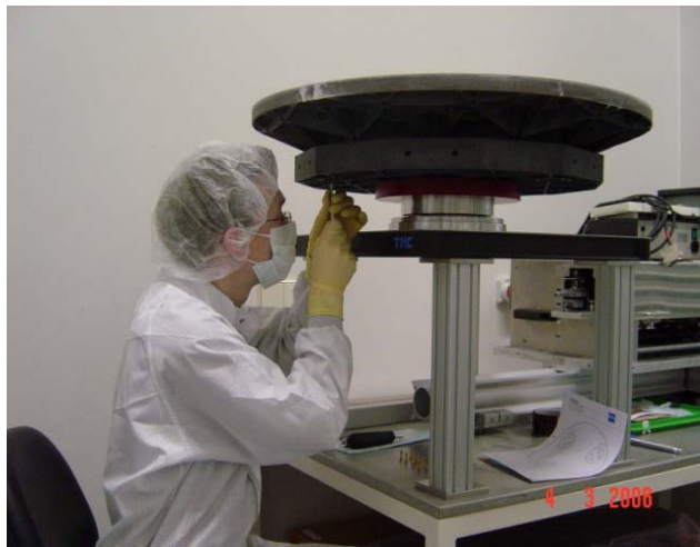
Fig.13 : Mirror during assembly to optical bench for optical measurement
