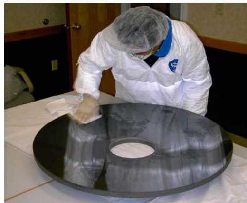
Fig.12 : pre-polished mirror during wipe test
