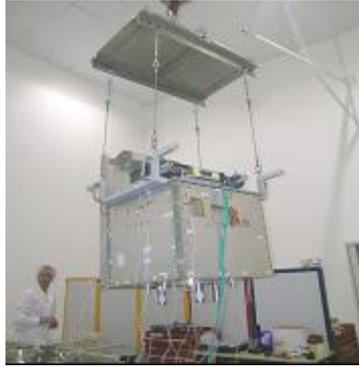
Fig. 10 FM flight telescope structure under shock tests
