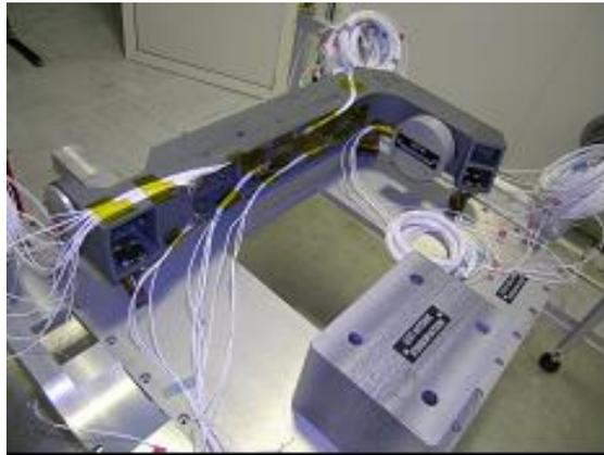
Fig. 8 FM structure equipped for vibration tests
