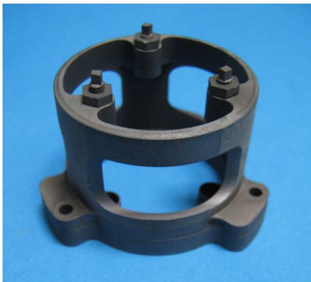
Etalon cage with M3 screws to fix the optic
