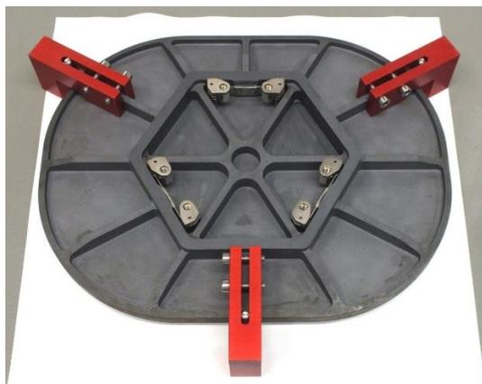
Fig 5. Backside of the mirror during integration with mounting clamps (Image DLR)
