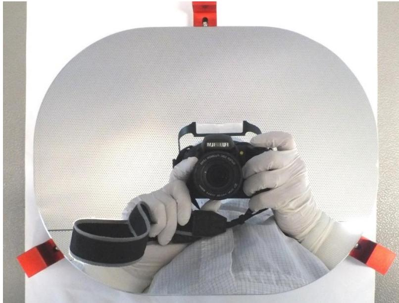
*Fig 6. Frontside of mirror during integration - (Image DLR)*
